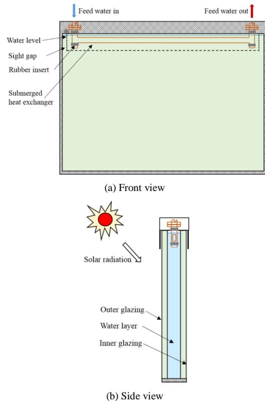
Figure 1. Water-filled double-glazing with submerged heat exchanger
