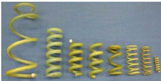
Fig. 4 Epoxy/E-glass fibre composite coil spring.
