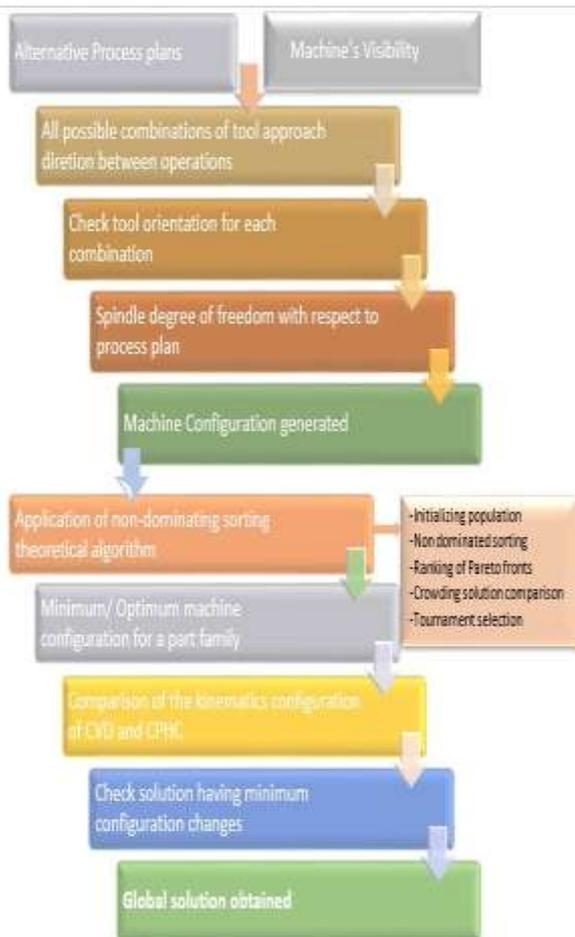
Figure 1. Algorithm for Optimal Machine Configuration
