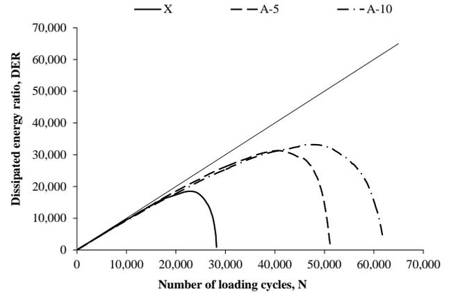
Figure 3. Evolution of DER as a function of loading cycles for blends with increasing crumb rubber dosage (example)
