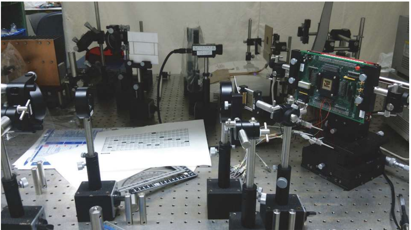
Fig. 3 Configuration experiment for an optically reconfigurable gate array.
