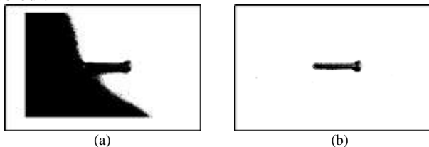
Figure 1. Comparison between global threshold and adaptive threshold. (a) Global threshold segmentation. (b) Adaptive threshold segmentation.
