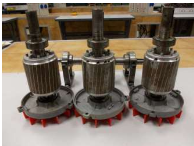
Fig. 4. Picture of the three rotors tested; healthy motor (left), motor with four broken bars (center), and motor with two broken bars (right).
