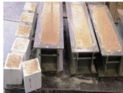
Figure 2. Fresh SFRC in beams and cubes moulds
