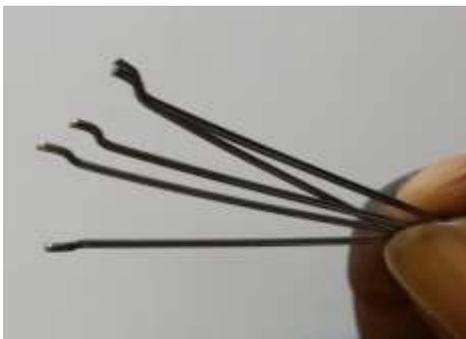
Figure 1. Hooked end steel fibres
