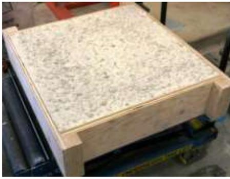
Figure 3. Casting of slab specimen
