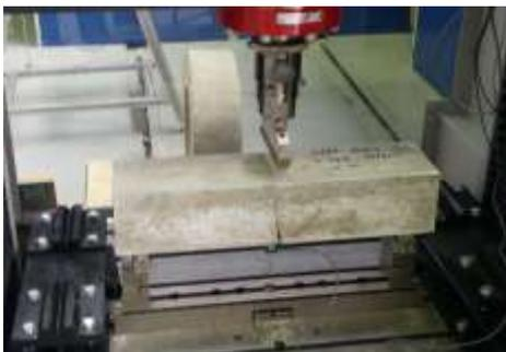
Figure 4. Three-point loading test of beam specimen
