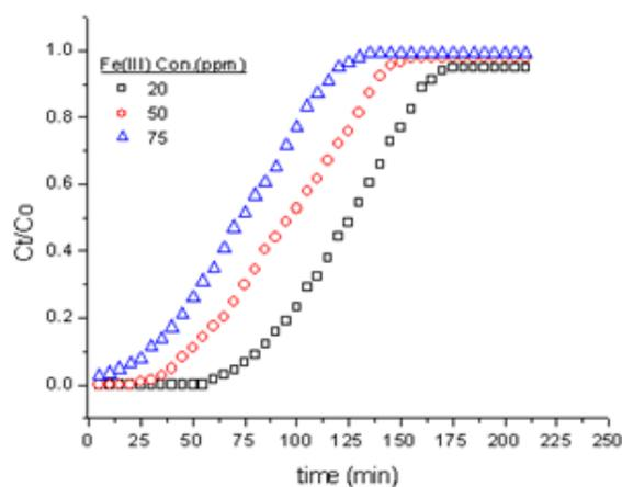
**Fig 1.** Experimental breakthrough curves of  $Fe^{+3}$  as a function of inlet  $Fe^{+3}$  concentration (T 15°C, pH 4, flow rate 5 mL.min<sup>-1</sup>, bed depth 5cm, particle size 0.25-0.5 mm)
