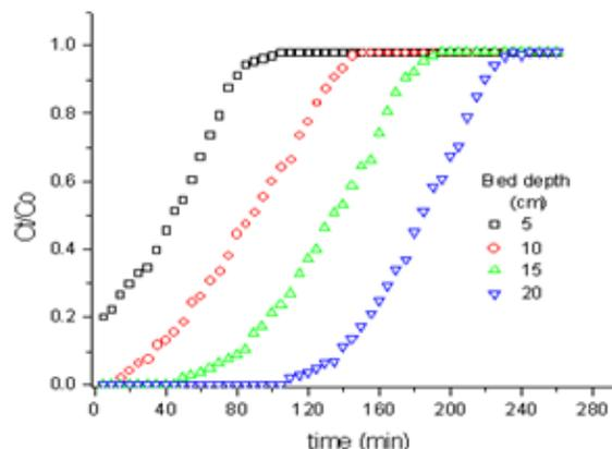
**Fig 3.** Experimental breakthrough curves of  $Fe^{+3}$  as a function of bed depth (T 15°C, pH 4, Co 50 ppm, flow rate 5 mL.min<sup>-1</sup>, particle size 1-2 mm).
