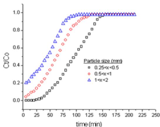
**Fig. 6.** Experimental breakthrough curves of  $\text{Fe}^{+3}$  as a function of particle size ( $T$   $15^\circ\text{C}$ , bed depth 5 cm, Co 50 ppm, flow rate  $5 \text{ mL}\cdot\text{min}^{-1}$ , pH 4).
