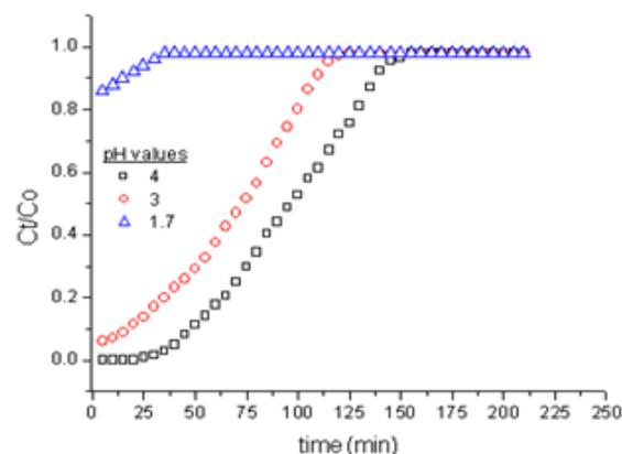
**Fig. 5.** Experimental breakthrough curves of  $\text{Fe}^{+3}$  as a function of pH of solution ( $T$  15°C, bed depth 5 cm,  $C_o$  50 ppm, flow rate 5  $\text{mL}\cdot\text{min}^{-1}$ , particle size 0.25-0.5 mm).
