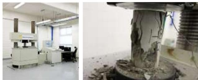
Figure 7. Compressive test of concrete with 3D fiber
