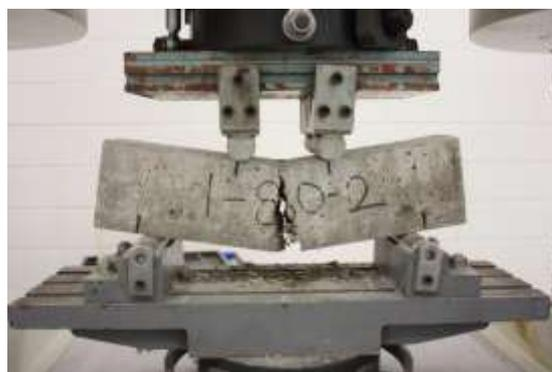
Figure 8. Flexural test of concrete with 3D fiber
