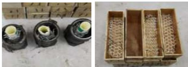
Figure 6. Specimens for the compressive and flexural strength test of concrete with 3D UHMWPE fiber
