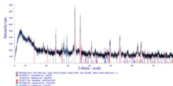
Figure 1. X-ray diffractogram of red mud from KAP
