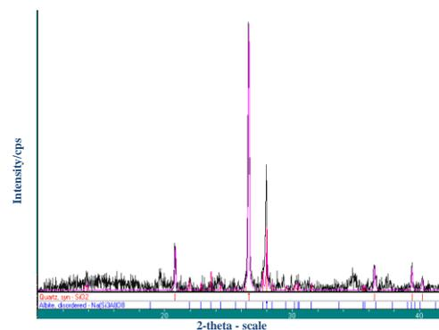
Figure 2. X-ray diffractogram of volcanic tuff "Jugoštica"
