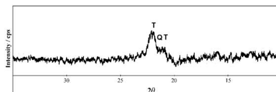
Figure 3. X-ray diffractogram of volcanic tuff "Strmoš"
