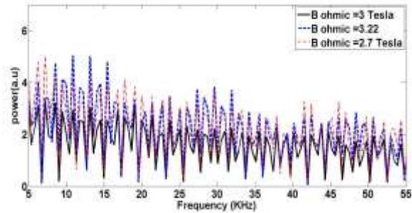
Figure 6. FFT of oscillations detected by Mirnov coils positioned at equatorial outer side mid-plane for plasma discharges  $B_{ohmic}$  with  $B_{ohmic} = 2.7\Omega$ ,
