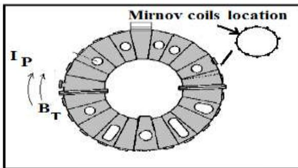
Figure 2. Schematic drawing of IR-T1 and locations of Mirnov coils .
