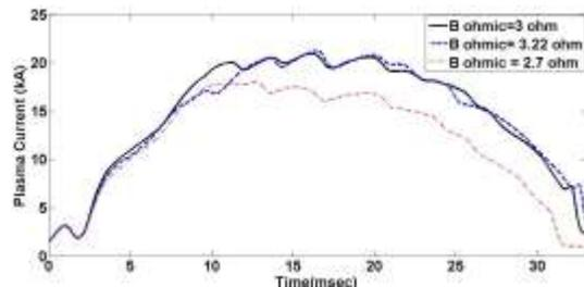
Figure 3. The time evolution of plasma current in the presence of  $B_{ohmic}$  with  $B_{ohmic} = 2.7 \Omega$ ,  $B_{ohmic} = 3 \Omega$ ,  $B_{ohmic} = 3.22 \Omega$
