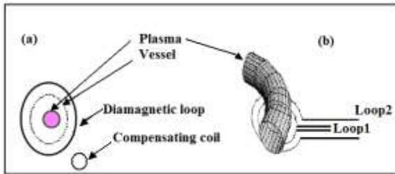
Figure 1. (a) Diamagnetic coil and compensating coil, (b) Two concentric magnetic loops
