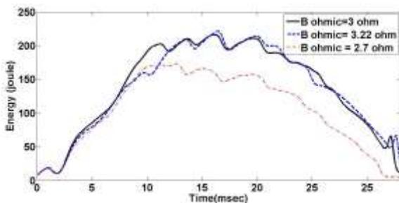
Figure 5. The time evolution of plasma energy in the presence of  $B_{ohmic}$  with
