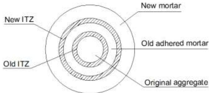
Figure 1 Five-phase composite sphere model, own elaboration from [2].
