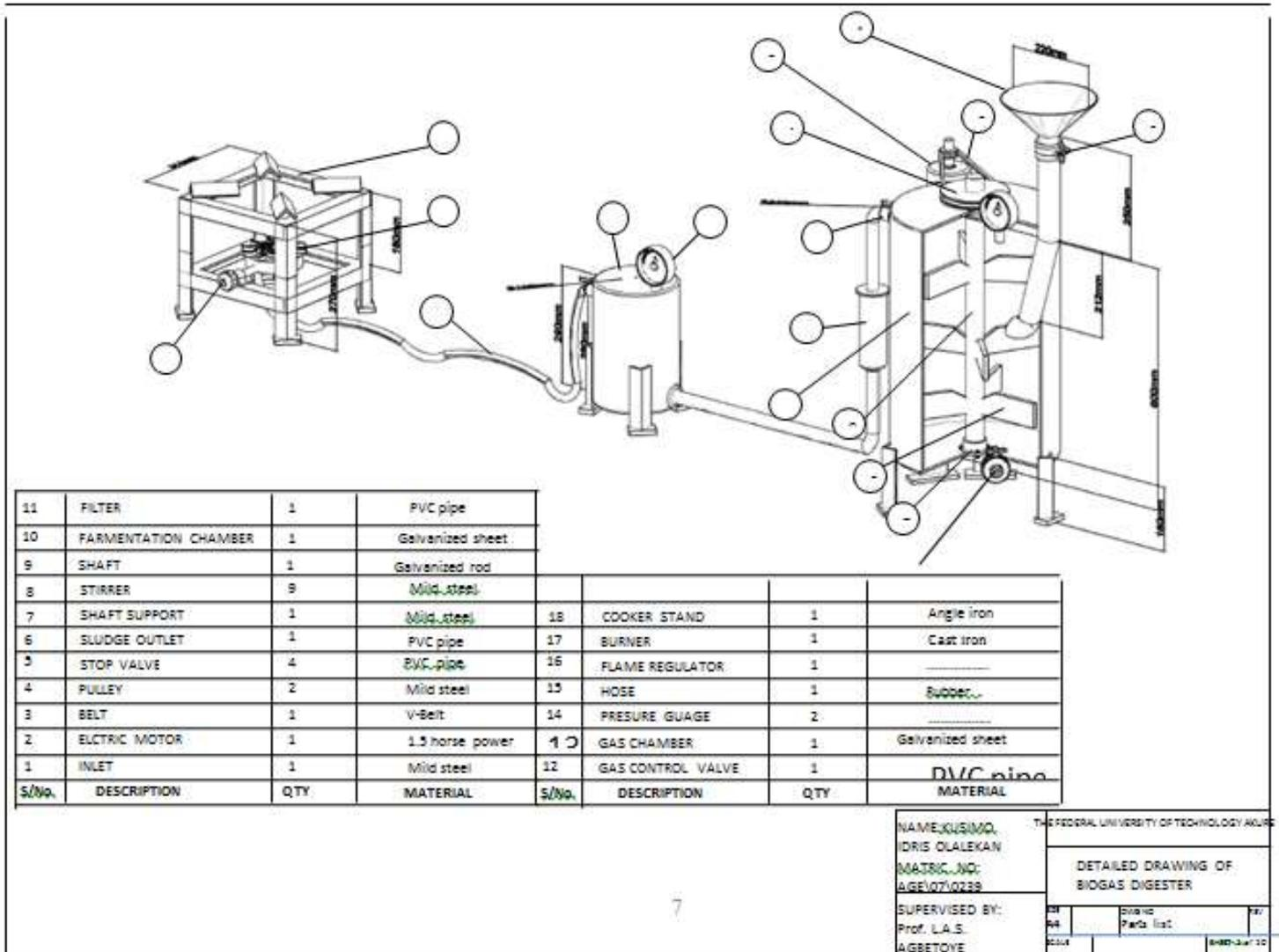
Figure 1: Exploded views of the Biogas production unit`
