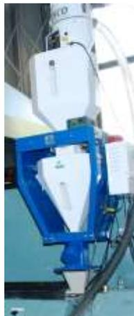
Fig. 2 Loss - in - weight hopper
