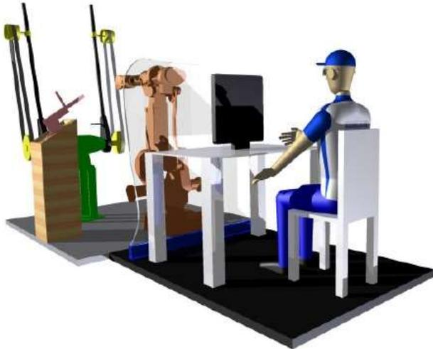
Figure 3 Education concept by OLP method. Working in an office environment, the user can generate robot programs without interrupt production. [7]
