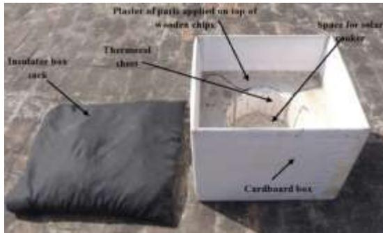
Figure 4: Photograph of insulator box with sack
