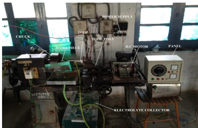
Figure 1 Electrochemical Honing Setup
