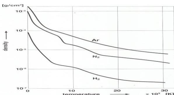
Fig. 1 Densities of argon, nitrogen and hydrogen plasma versus temperature (p = 1 bar)
