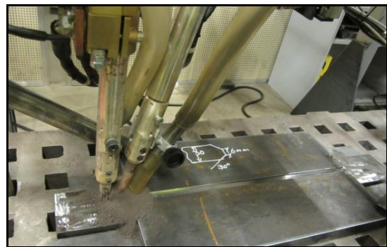
Figure 3. Tandem Single + ICE@ welding system configuration [5]
