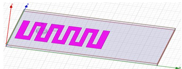
Figure 1(b) Meandered Planar Inverted F Antenna (PIFA)
