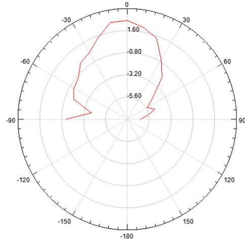
Figure 3(a) Radiation Pattern at Frequency 8 GHz, phi=60°
