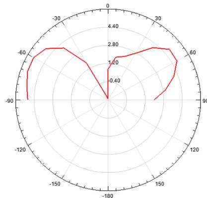
Figure 3(c) Radiation pattern at frequency 3.8 GHz, phi=60°
