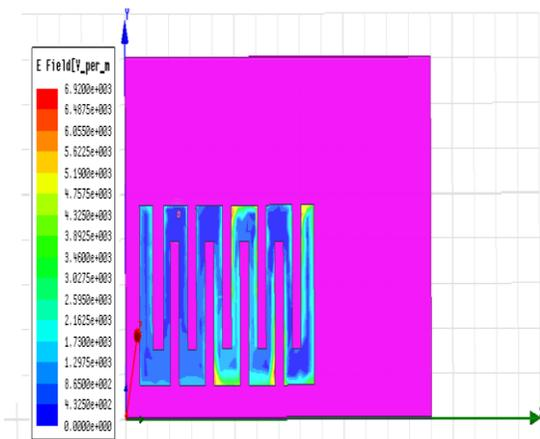
Figure 5 Electric Field Distribution on Radiating Patch (V-per-m)
