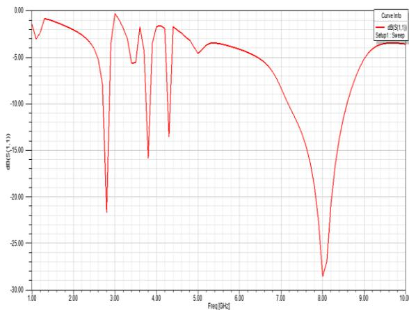
Figure 2 Simulated Magnitude of the S<sub>11</sub> Parameters of Proposed Antenna
