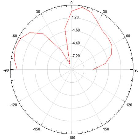
Figure 3(b) Radiation Pattern at Frequency 2.8 GHz, phi=60°
