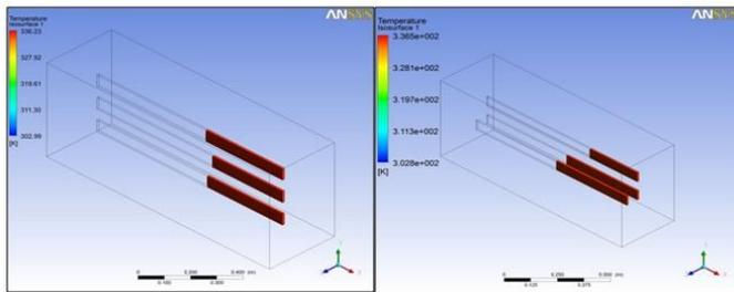
Figure 5. Isotherms for vertical and L-shape configuration
