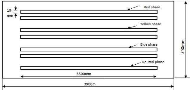
Figure 6. Schematic of substation bus-bar
