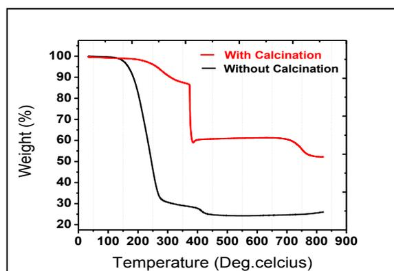
Figure 5. TGA thermograph of MoS<sub>2</sub> nanoparticles.
