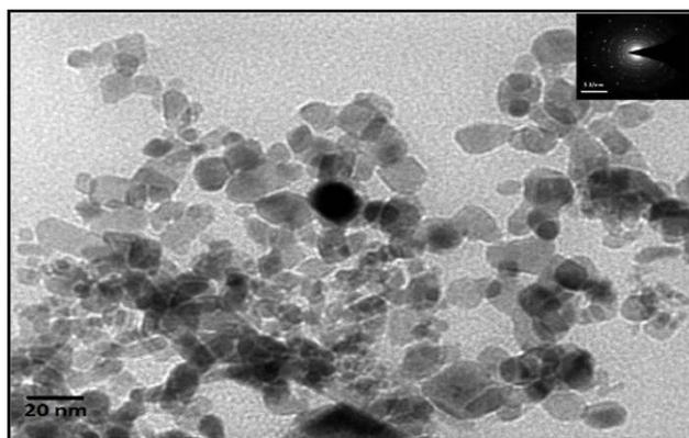
Figure 2. MoS<sub>2</sub> nanoparticles.
