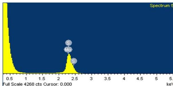
Figure 4. EDX pattern of MoS<sub>2</sub> nanoparticles.
