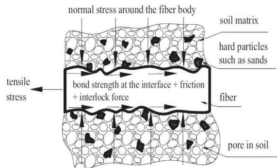
Fig. 1.7 Interaction between soil particle and fiber [4]
