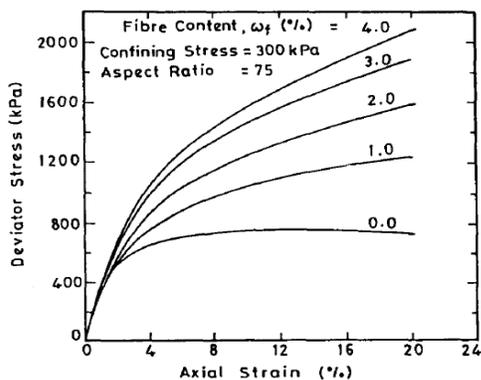
Fig. 1 Stress strain behaviour of fiber reinforced sand for different fiber content [14]
