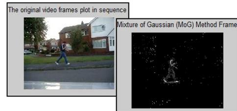
Fig.4 Background Subtraction using Mixture of Gaussian
