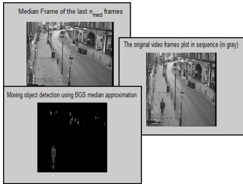
Fig.2 Background Subtraction using Approximate Median
