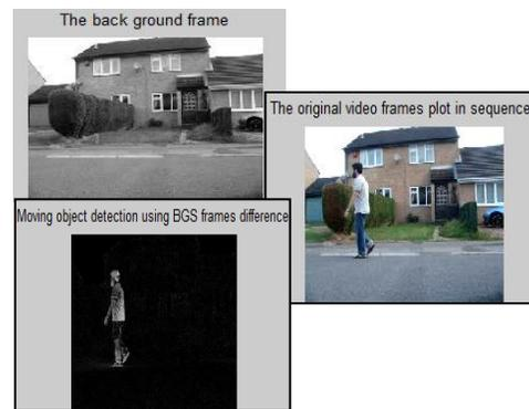
Fig.1 Background Subtraction using Frame Difference
