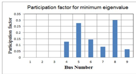
Figure 4 The participating factor of all buses for most critical mode of the test system
