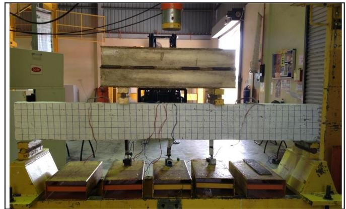
Figure 4. Flexural capacity test setup
