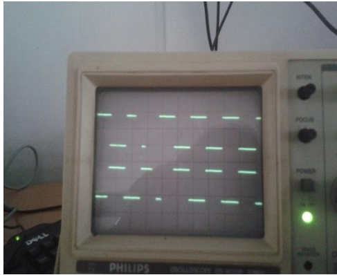
Multilevel PWM single phase experimental results using at M_a < 0.5
