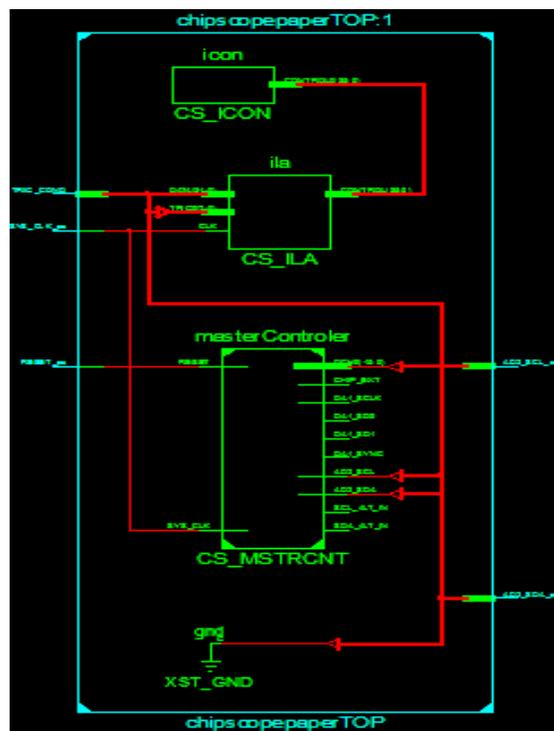
Figure 4. Internal view of Register Transfer Level (RTL) Synthesis result showing interconnection of “masterControler”, “icon”, “ila” modules within the top level entity “chipscopepaperTOP”.
