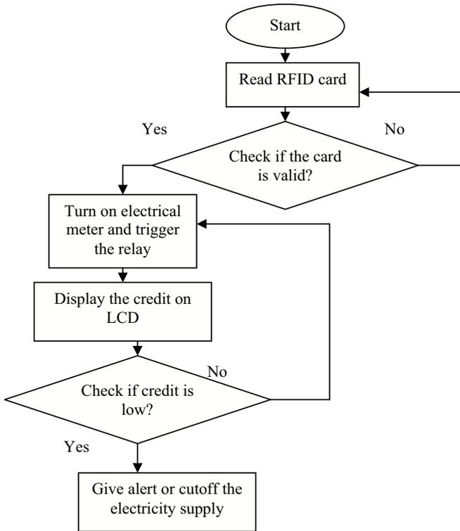
Figure 2. The main program design to control the electricity turn ON/OFF.
