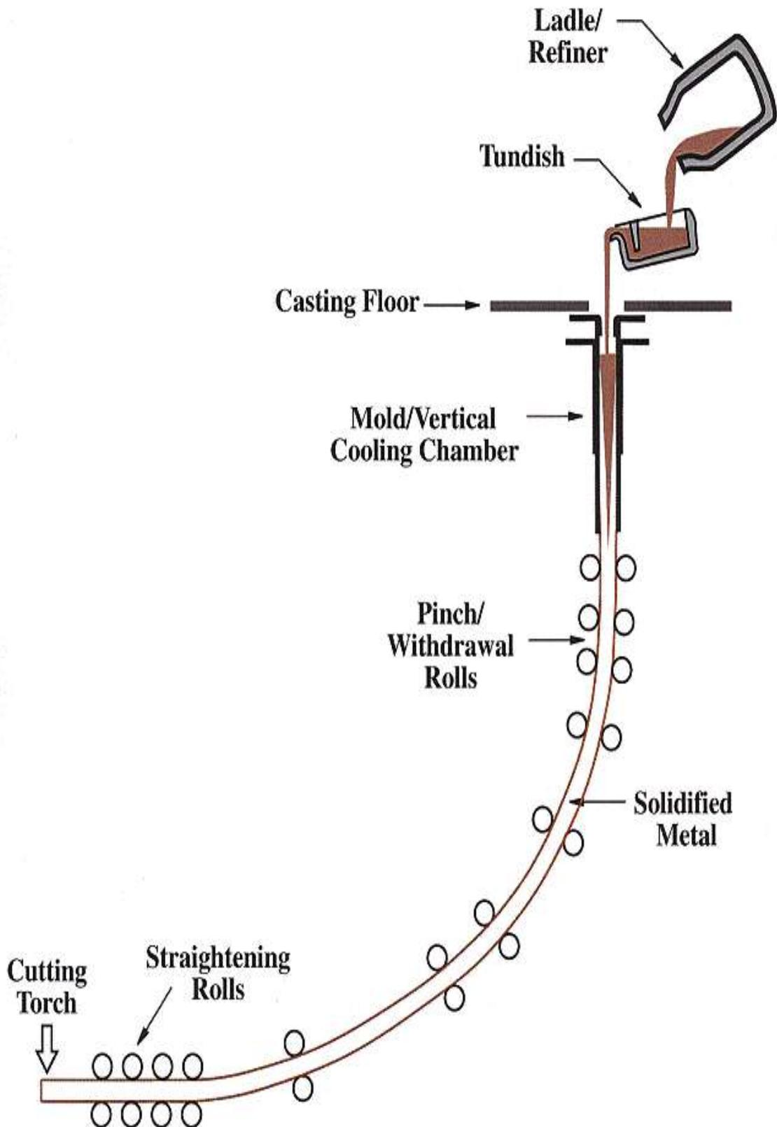
Figure-3 (b) Schematic Sketch of Continuous Casting Process with Straightening Rolls and Cutting Torch
