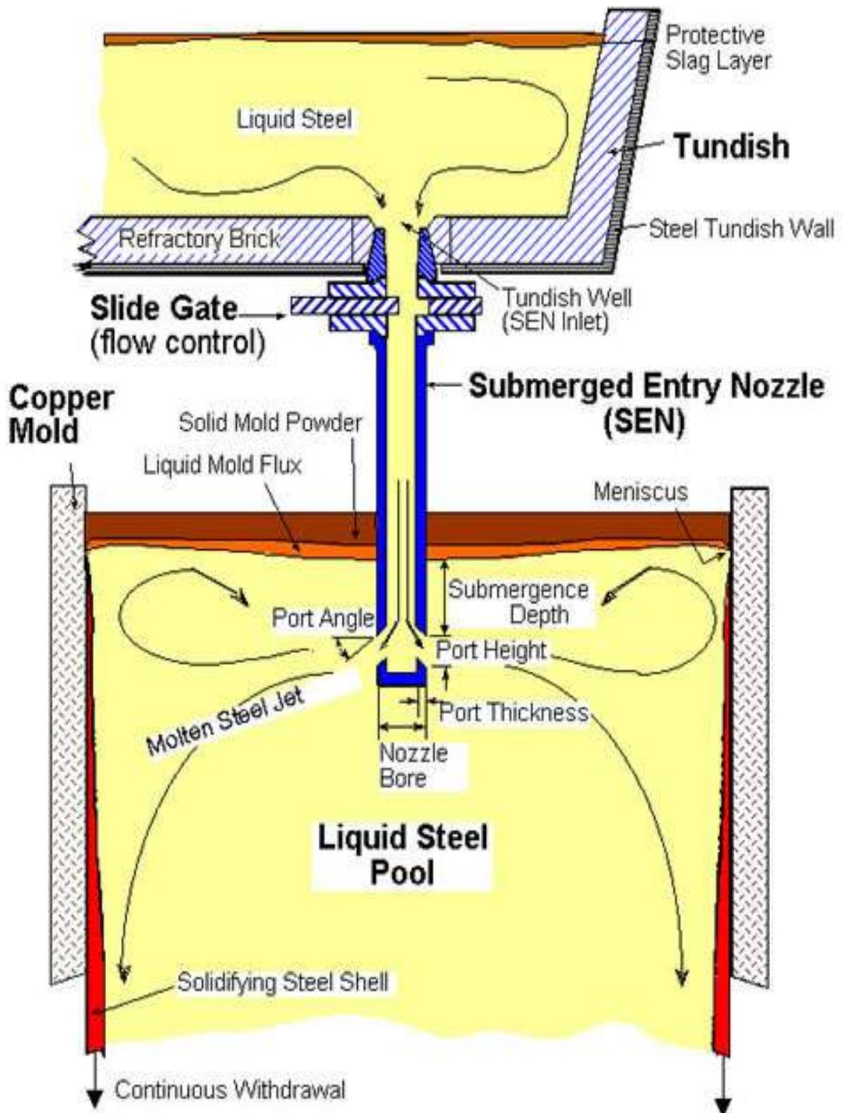
**Figure-5(a) Mechanism of Continuous Casting Process**
